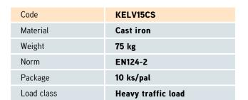
without hinge, PUR shock-absorbing lining - tunnel version, without spring-loaded lid locking in frame, watertight to 2 bar
